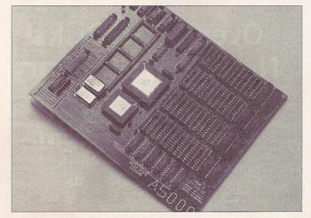
There are two distinct types of faster processor, the 68020 and the 68030. A typical speed for the 68020 is 16-25 MHz, while the 68030 goes at 16-50Mhz. The speed of the processor is built into the accelerator board at the factory. So go for the raw speed - 68030 boards cost more but they are faster and usually have a greater capacity for extra 32-bit memory (memory only usable by a faster CPU, much faster than standard memory for various reasons).
