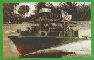
Well sir, your PBR is a military conversion of a commercial craft designed 25 years ago. Three generations of PBRs have lead to the post-Vietnamese war Mark III that you see before you. Achieving 50 knots from twin 450-horsepower engines, this baby can brake down from top speed to a dead stop in less than one boat length.
